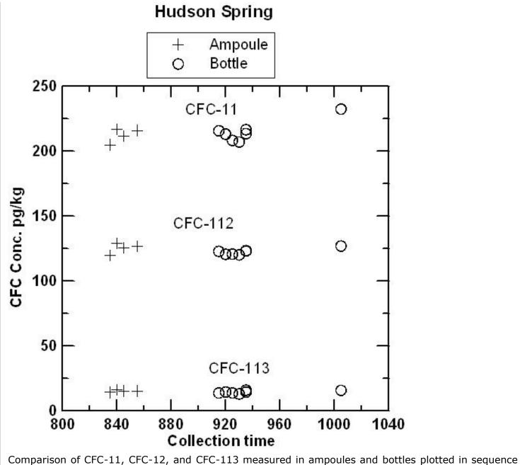
Comparison of CFC-11, CFC-12, and CFC-113 measured in ampoules and bottles plotted in sequence of field collection. The plot suggests that at least some of the very small variations observed represent real variations in water composition discharging from the spring, rather than changes occurring during storage.
